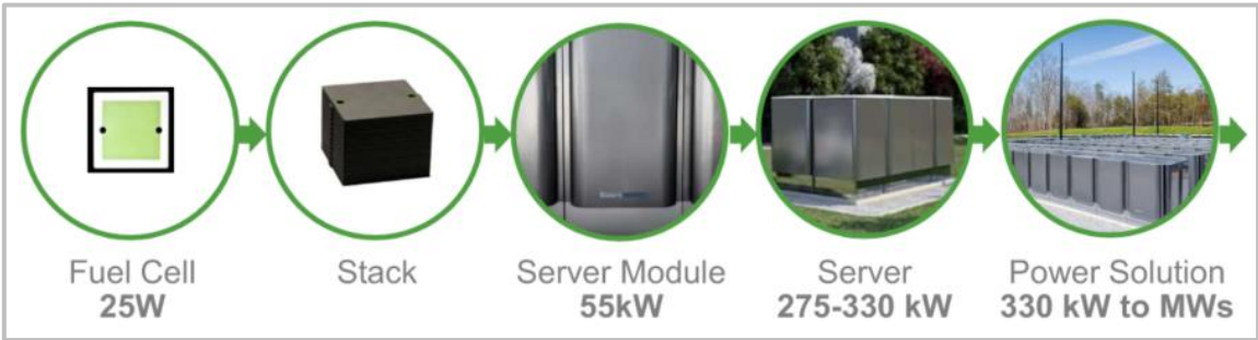
Figure 8: A Fuel Cell Power Solution
