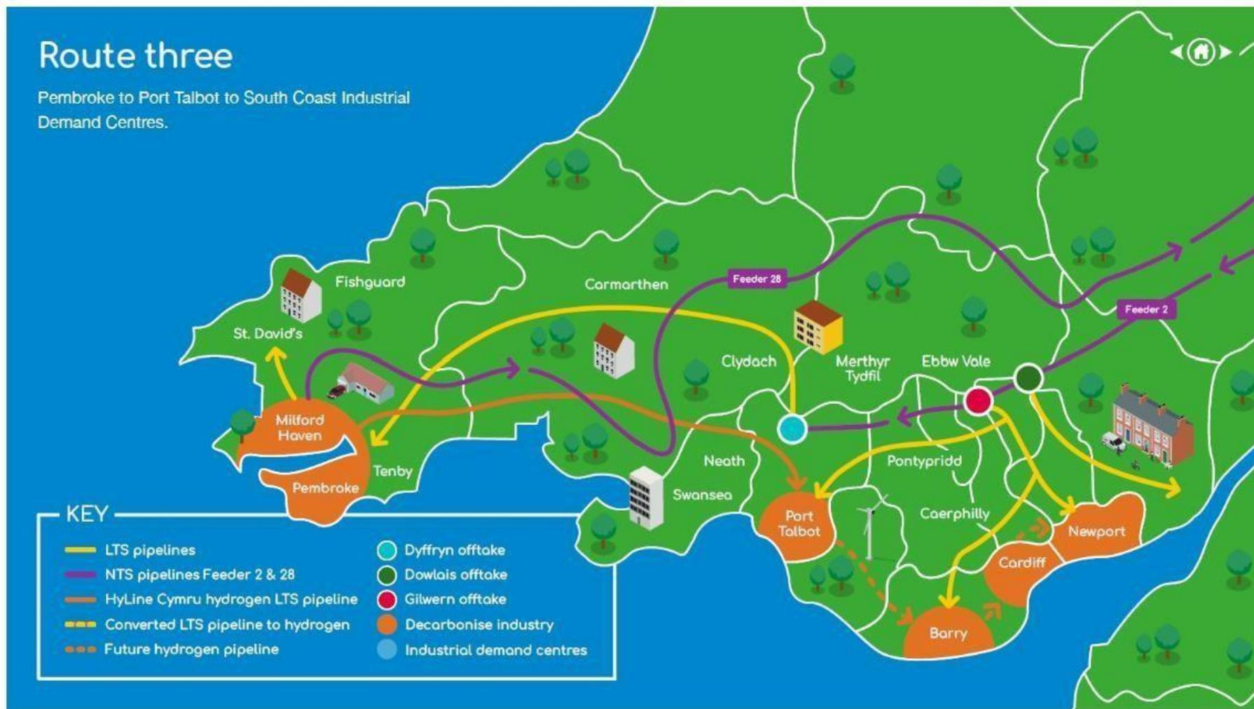
Figure 17 Routing options considered for HyLine Cymru pipeline R2
