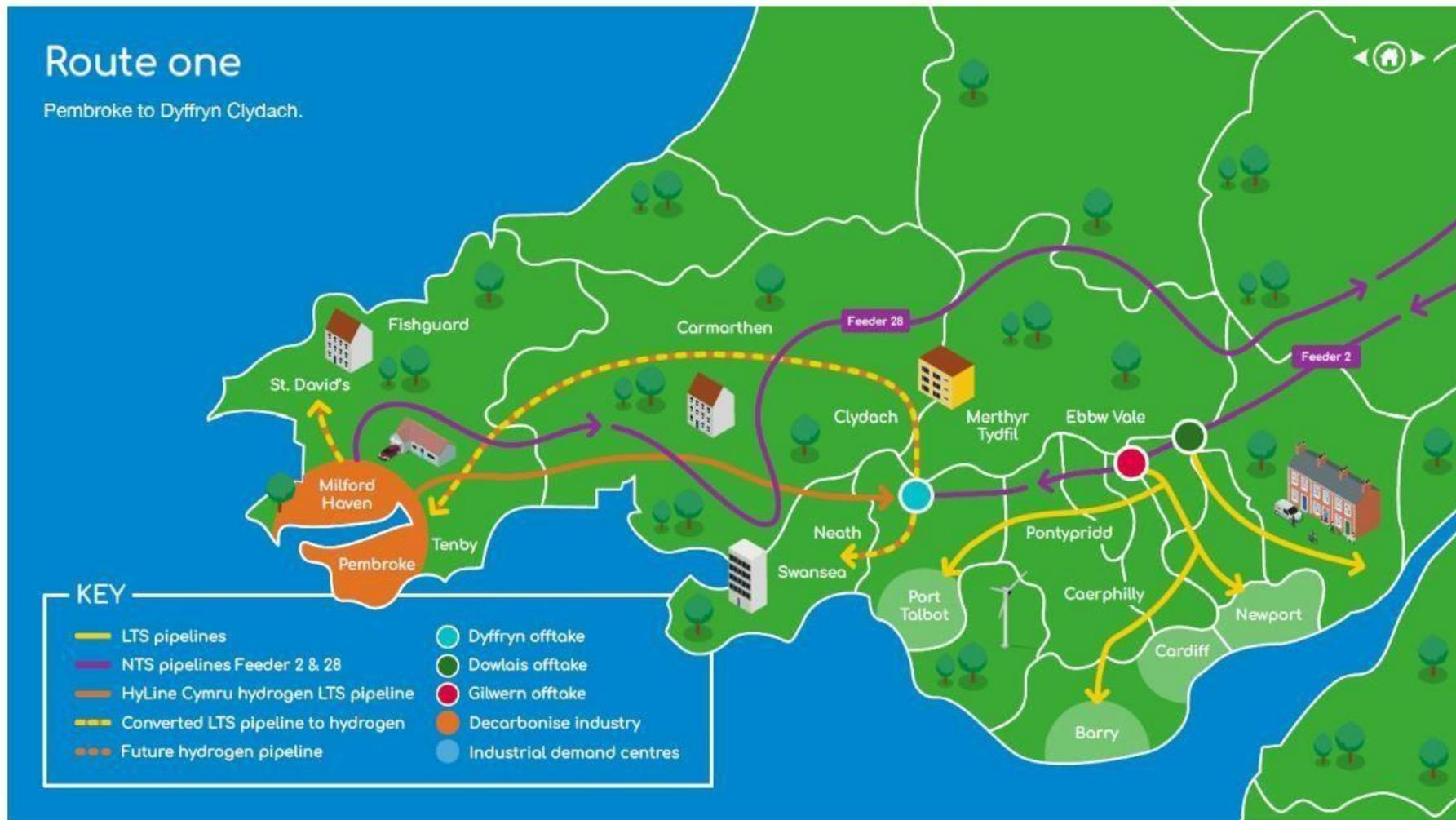
Figure 15 Routing options considered for HyLine Cymru pipeline R1
