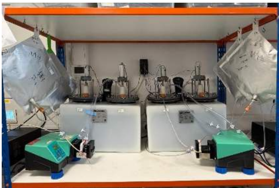
Figure 2: Experimental set up of Laboratory digester system used for hydrogen-assisted anaerobic digestion experiments.
