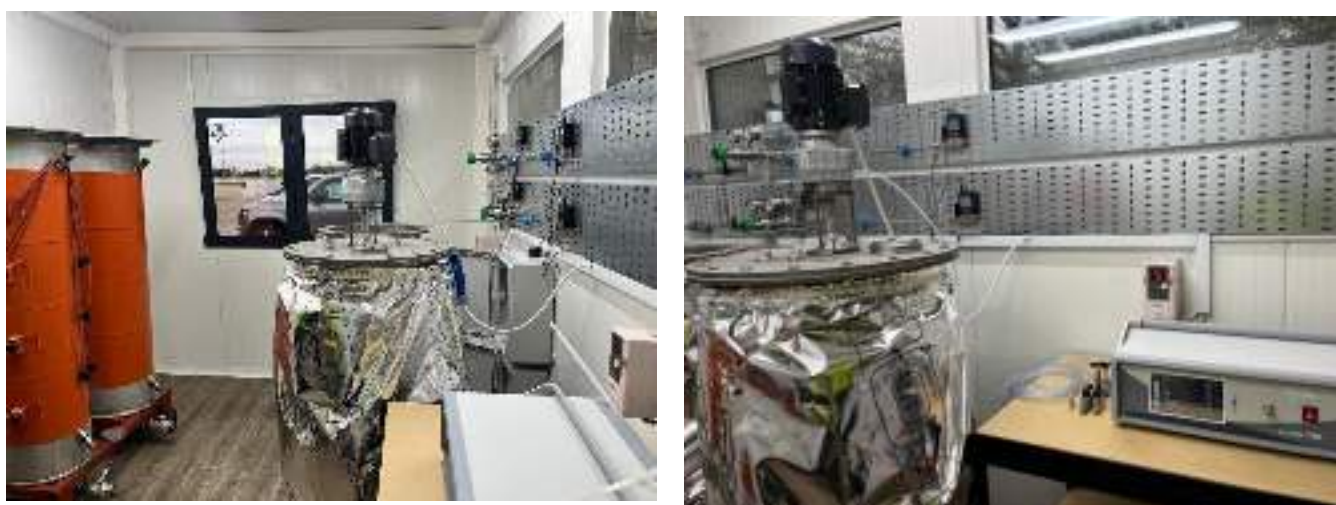
Figure 9: Experimental Set up within a containerised mobile laboratory installed within the AD facility.
