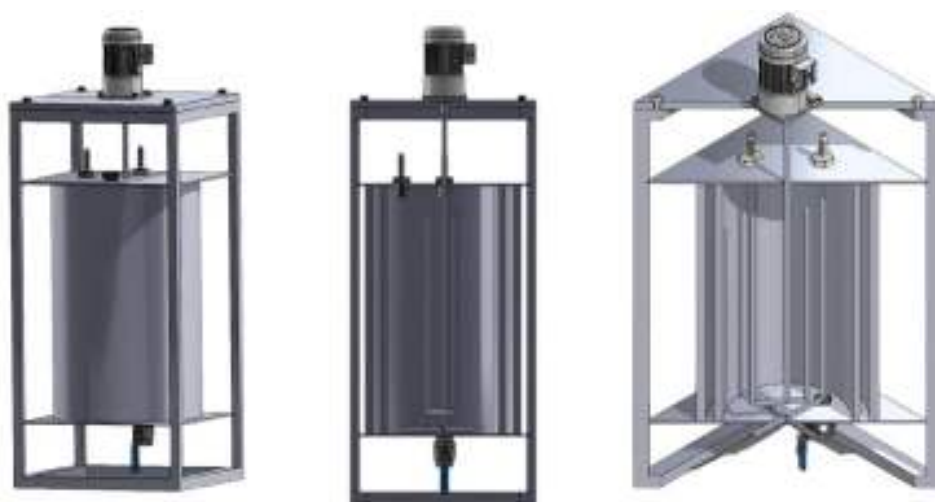
Figure 8: CAD representations of the anaerobic digestion test reactor vessels used within the on-site testing programme.
