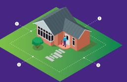
Permanent or temporary buildings must not be constructed over our pipes or within the minimum building proximities. Where there is an easement – a legal agreement for our mains to be on private land – there may be further restrictions to working near our pipes.
