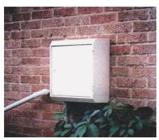
(A) SURFACE MOUNTED METER BOX This is installed by our teams when we arrive on site. The box cannot be positioned above or within 150mm of the edge of drains, inspection covers, manholes, air bricks, etc. Height: 497mm, Width: 442mm, Depth: 230mm.
